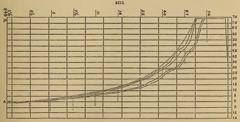
like the one shown in Fig. 4212, or most economical, like Fig. 4213. For the purpose of ascertaining the power exerted, we have merely to measure its included area, and so get the mean
